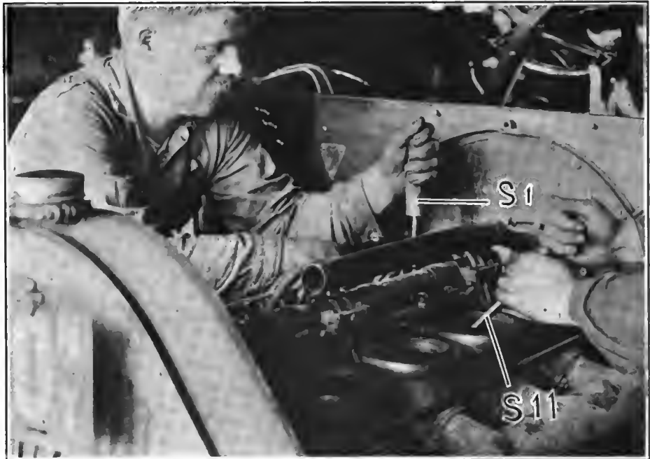
Fig. 4—A frequent operation—grinding valves and scraping out carbon
